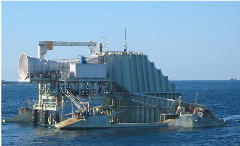
Figure 8: OceanLinx OWC Wave Energy Converter
